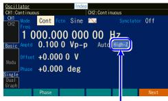
Select the load impedance icon and then press the ENTER key
