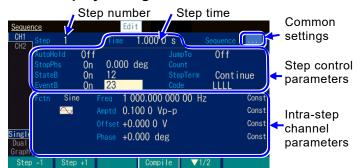
The step control parameters of one step and the intra-step channel parameters of one channel are displayed simultaneously.
