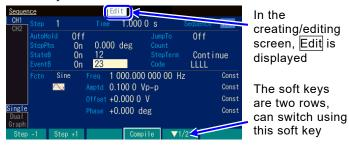
During editing, the waveform of the selected step is output to the waveform output.
