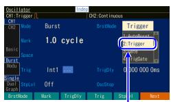
Select 'Trigger' in "BrstMode" and then press the ENTER key
