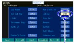
In the Utility screen, select "ΦSync" and then press the ENTER key to execute the phase synchronization
