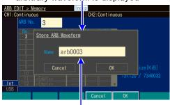
Enter a name for the arbitrary waveform, select the [OK] soft key, and press the ENTER key, the waveform data is saved
