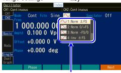
The selection list for the polarity/ amplitude range is opened
