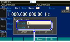
Set the ratio in the input fields of "Ratio(N)" and "Ratio(M)"
