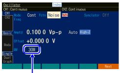
Set the equivalent bandwidth so that the bandwidth and amplitude density of the noise become optimal
