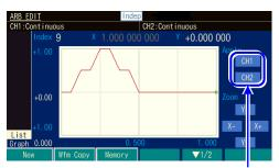
Select [CH1] or [CH2] and press ENTER to output the waveform. For WF1983/WF1981, press [Apply]
