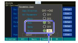
Copy the modulation and burst parameters
