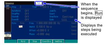
The screen displays the step being executed (horizontally scrolls when displaying a Graph).
