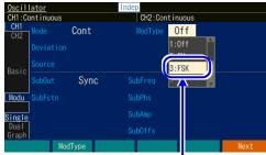
Select the modulation type "ModType" ( P.4-14) on page 4 "Modu" of the setting screen. Set the option that appears to 'FSK'. P.4-18 You can also use the numeric keypad 3.
