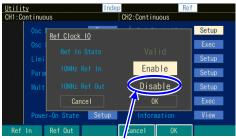
Frequency reference output is turned on when this is 'Enable' and turned off when it is 'Disable'
