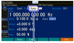
The waveform is set to 'Ramp'
