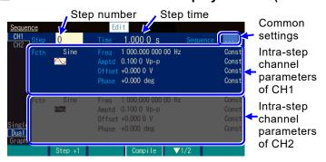
The intra-step channel parameters of one step are displayed for two channels simultaneously. For the step control parameters, only the step time is displayed.
