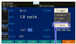
Select burst mode "BrstMode" ( P.4-14) on page 3 "Burst" of the setting screen to display the burst mode selection list.
