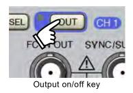
The output terminal is released when the output is turned off.
