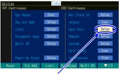
In the Utility screen, select the "User Unit" field and press the ENTER key
