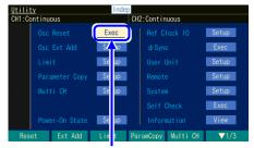
In the Utility screen, select "Osc Reset" and press the ENTER key
