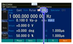
When the waveform is set to pulse, the edge selection icon appears
