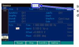
In the hold state, Hold is displayed Press the [Hold] soft key in the Run state to pause the sequence. The sequence goes into standby while keeping the output condition as is.
