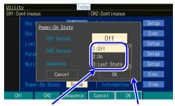
Set the output The dialog for settings setting condition at power-on opens
