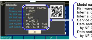
Model name serial number Firmware version Internal device information Internal device information Service data Date and time last adjusted by NF Corporation Date and time last calibrated by NF Corporation
