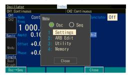
When the MENU key is pressed, the top menu opens. Select "Utility" and then press the ENTER key. The Utility screen opens. You can also use the numeric keypad 3 after the top menu is displayed.
