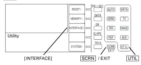
[INTERFACE] Switches to the {interface configuration screen}.
