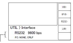
Current settings: Data rate/flow control, terminator
