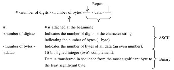
When transferring multiple numeric data, the data is transferred continuously without delimiters (such as commas).
