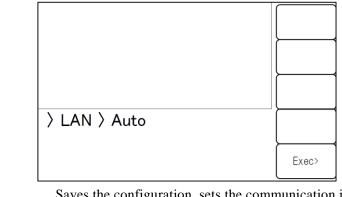
[Exec] Saves the configuration, sets the communication interface to LAN, and returns display to the {LAN configuration screen}.
