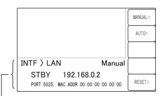
Current statuses: LAN status / IP address / IP configuration method (manual or auto)
