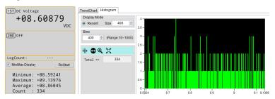
2. If we set "10" in the field, the histogram shows us the maximum bins is decreased to 10 and each bin has more measured counts than the previous. Also, the highest measured counts of bin are 36 in Y scale.
