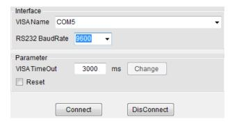
5. The VIS TimeOut allows user to define a period before timeout. From the figure below where the default 3000ms indicates if there's no response from the DM2571 over the set 3000ms (max. 60000ms), the measurement will be halted accordingly.
