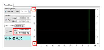
1ST & 2ND Y Scale Trend chart supports dual channels display simultaneously. The Y scale, therefore, is divided into 1ST and 2ND sections. The way to define 2ND Y scale is identical with that of the 1ST display as mentioned above. Refer to the following figure in which red highlight indicates the Y scale of the 1ST display, whereas orange indicates the Y scale of the 2<sup>ND</sup> display.
