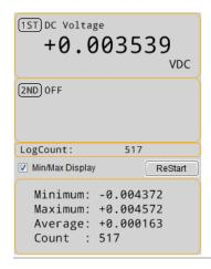
When the 2ND display is enabled, the measured Note value will be shown in 2ND section and the **Min/Max Display**, however, will be deactivated.
