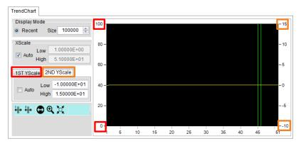
Note The 2ND Y Scale section hides out when the 2ND display measuring function is disabled.
