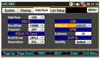
Press the F5 (Enter) key or Knob key followed by scrolling Knob key or pressing +/- keys to land on the desired USB Protocol option. We adopt USB-CDC in the example here.
