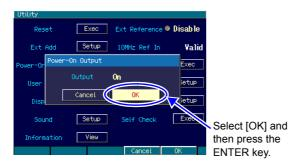
4. Once the desired power-on output setting has been completed, select [OK] in the lower part of the window and then press the ENTER key. The power-on output setting change is applied and the window closes.
