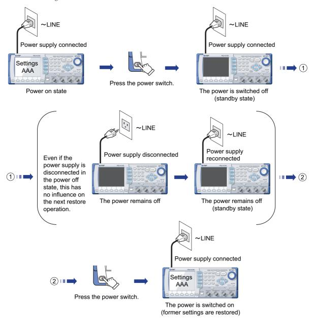
While the equipment power is off, even if the power supply is cut off due to the disconnection of the cord or the shutoff of a connected breaker, this has no influence on the restore operation the next time the equipment is powered on again.
