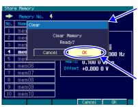
Press the [Clear] soft key to open the dialog box for checking the initialization operation
