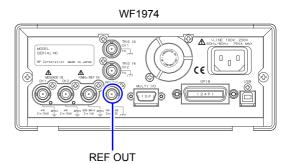
Use REF OUT to unify the frequency and phase for multiple WF1973, WF1974 units. Connect the frequency reference output of the master unit when multiple units are combined in synchronous connection, or the master WF1973 or WF1974, to the external 10 MHz frequency reference input of the WF1973 or WF1974.
