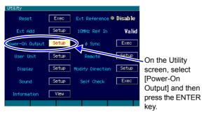
2. On the Utility screen, select the [Power-On Output] field and then press the ENTER key.
