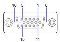
Figure 3-5. Multi-I/O Connector Pin Assignment
