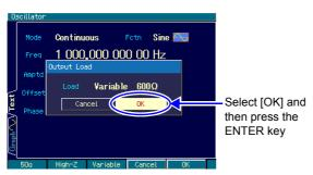
3. Once the load impedance setting has been completed, select [OK] in the lower part of the window and then press the ENTER key to apply the load impedance setting change and close the window.
