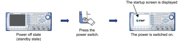
Once the power is switched on, a self-check test is automatically executed and the unit becomes operable.
