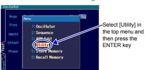
1. Press the MENU key to open the top menu window. There, select [Utility] and then press the ENTER key to display the Utility screen.
