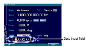
1. Select the [Duty] field and then press the ENTER key to open the duty input field.
