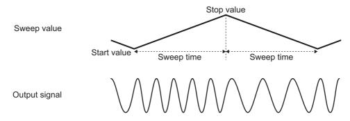
As the phase increases, the frequency rises by the value below, and as the phase decreases, the frequency drops by the value below.
