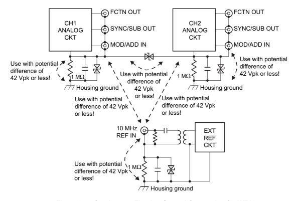
Figure 3-7. Cautions on Floating Ground Connection for WF1974
