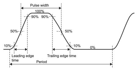
However, the setting ranges of the pulse width, leading edge time, trailing edge time, and frequency are mutually limited as follows.
