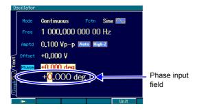
1. Select the [Phase] field and then press the ENTER key to open the phase input field
