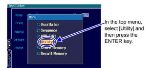
1. Press the MENU MENU key to display the top menu window. In that window, select [Utility] and then press the ENTER key to display the Utility screen.
