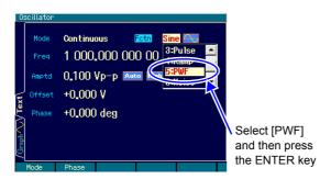
Select the [PWF] parameter-variable waveform in the [Fctn] field and then press the ENTER key.
