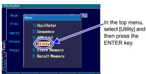
1. Press the MENU MENU key to display the top menu window. In this window, select [Utility] and then press the ENTER key to display the Utility screen.
