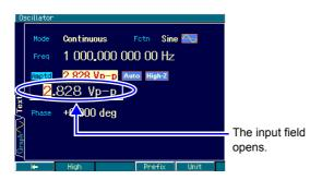
**1.** Select amplitude and then press the ENTER key to open the input field.
