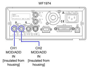
When the modulation source is external, except for FSK and PSK, an external modulation signal is input. In the case of the FSK and PSK, the external trigger input is used as external modulation signal input.
