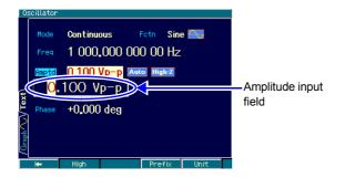
1. Press the AMPTD shortcut key to open the amplitude input field. Alternatively, select the [Amptd] field and then press the ENTER ENTER key to open the amplitude input field.
