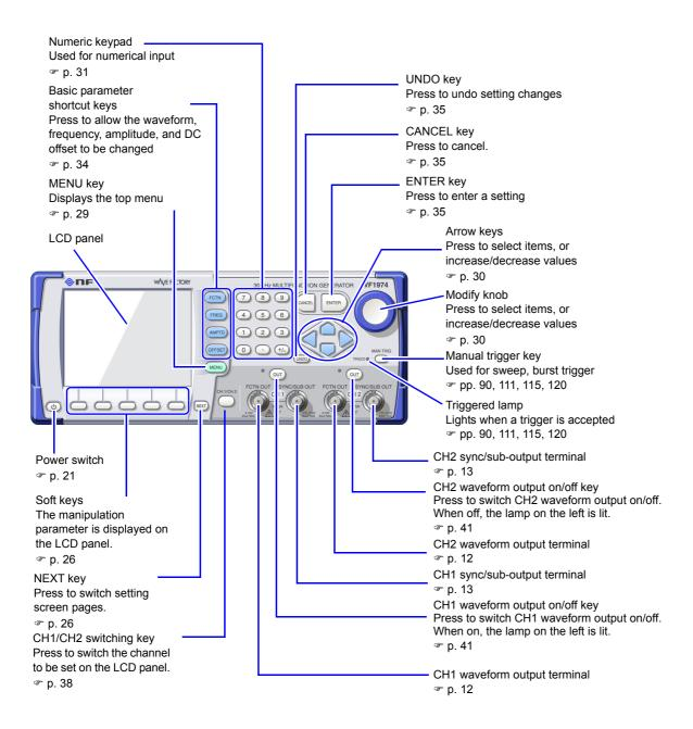
Figure 3-3. Front Panel of WF1974
