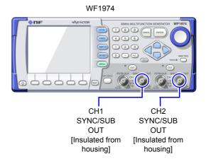
A sync signal is output according to the waveform or oscillation status. This signal can be used as the oscilloscope synchronization signal.
