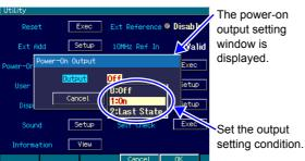
**3.** The power-on output setting window is displayed, so select the desired item and then press the ENTER ENTER key.
