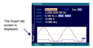
3. The Graph tab screen display is switched to by pressing the ENTER key. The settings can be done while checking the image of the output waveform on this screen.
