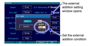
**3.** The external addition setting window opens, so select the desired item and then press the ENTER ENTER key.
