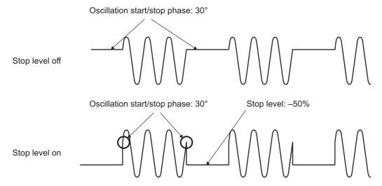
When the stop level is applied to a square waveform, a 3-value square waveform can be output, as shown in the following figure. In the example presented in this figure, the stop level is set to 0%, and the oscillation start/stop phase to 0°. (Either the normal or extended variable duty range may be used.) If the stop level is not applied, the level of the square waveform during oscillation stop is either to low level or high level.
