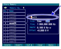
Press the [Rename] soft key to open the setting memory name input field  Similarly to the saving operation, after setting the setting memory number, press the [Rename] soft key to open the setting memory name input field.
