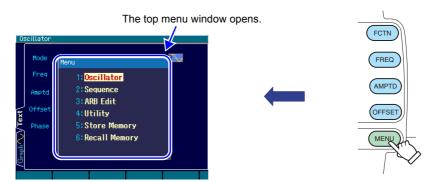
Select the desired menu item using the Q up/down arrow keys or the Q modify knob, and then press the ENTER key to display the menu item setting screen.
