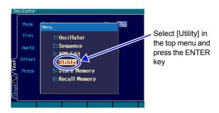
The top menu window is displayed by pressing the MENU key. In this window, select [Utility] and then press the ENTER key to display the Utility screen.
