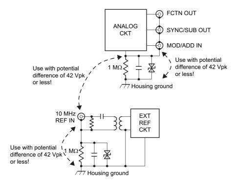
Figure 3-6. Cautions on Floating Ground Connection for WF1973
