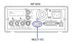
MULTI I/O can be used for sweep control and sequence control. It outputs the step synchronization code for the sequence.
