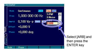
Select [ARB] (arbitrary waveform) in the [Fctn] field and then press the ENTER key.
