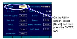
2. On the Utility screen, select the [Reset] field and then press the ENTER key. The settings are initialized.
