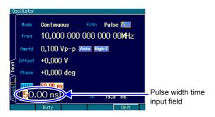
1. Select the [Width] field and then press the ENTER key to open the pulse width time input field.
