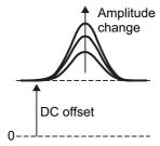
If the amplitude range is set to -FS/0, the amplitude changes using the top of the waveform as reference.
