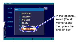
1. Press the MENU key to display the top menu window. In this window, select [Recall Memory] and then press the ENTER ENTER key to display the Recall Memory screen.
