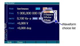
1. Press the FCTN shortcut key to display the waveform choice list. Alternatively, select the [Fctn] field and press the ENTER key to open the choice list.
