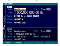
The channel to be set can be switched with the CH1/CH2 key.
