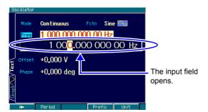
**1.** Select frequency and then press the ENTER key to open the input field.
