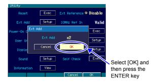
4. Once the external addition settings have been completed, select [OK] in the lower part of the window and then press the ENTER key to apply the external addition setting change and close the window.
