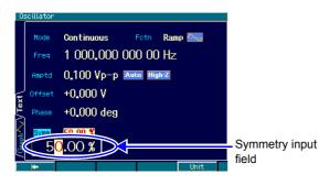
1. Select the [Symm] field and then press the ENTER key to open the symmetry input field.
