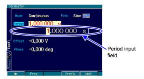
Once the period input field is opened, the setting procedure is the same as for the frequency.
