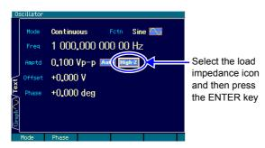
**1.** Select the load impedance icon on the right of the range icon and then press the ENTER ENTER key.
