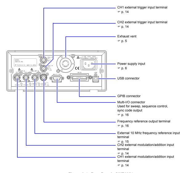
Figure 3-4. Rear Panel of WF1974
