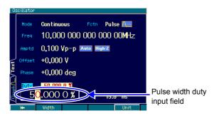
**1.** Select the [Duty] field and then press the ENTER key to open the pulse width duty input field.
