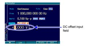
1. Press the FISE OFFSET shortcut key to open the DC offset input field. Alternatively, select the [Offset] field and then press the ENTER key to open the DC offset input field.
