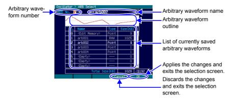
The changes are not reflected to the output waveform until applied by pressing the [OK] soft key (the operation differs from that for parameter-variable waveforms).
