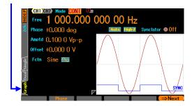
3. Press the ENTER key to switch to the Graph tab screen.
