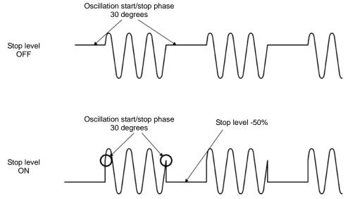
When you the stop level is applied to the square wave, a square wave with three values can be output as shown in the following figure.
