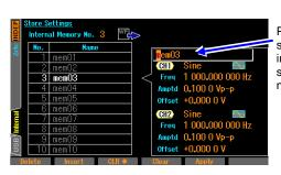
Press the [Rename] soft-key to open the input field of the setting memory name
