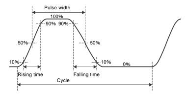
However, the setting range is restricted mutually as for pulse width, leading time, trailing time, and frequency as shown below.
