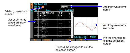
The changes will not be reflected in the output until the [OK] soft-key is pressed. Arbitrary waveforms cannot be created on this screen. For creation of arbitrary waveforms, data format and memory capacity, P. 7-2.
