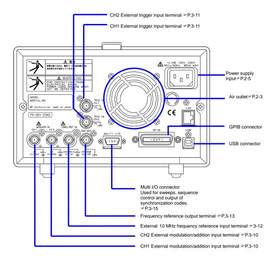
Figure 3-4 Rear Panel of WF1968
