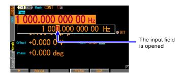
1. Select frequency and then press the ENTER key to open the input field.
