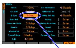
In the Utility screen, select [φSync] and then press the ENTER key to execute the phase synchronization
