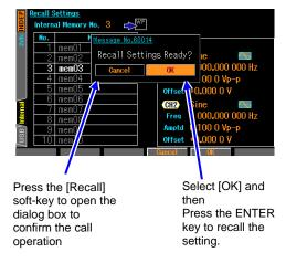
When the MENU key is pressed, the top menu opens. Then, select [Recall Settings]. This opens the Recall Settings screen.
