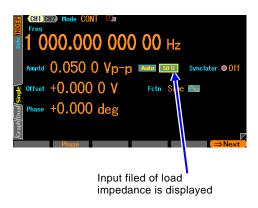
Select the desired load impedance condition, and then press the corresponding soft-key. When [Vari] is selected, the load impedance can be set. In this case, the input field of load impedance value is displayed to the right of the load impedance field.
