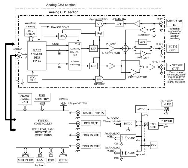
Figure 1-2 WF1968 Block Diagram
