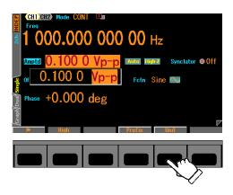
3. You can use the up/down keys or the modify knob to change the units to Vrms, dBV, or a user-defined unit (in the case of sine wave and load impedance Hi-Z). This just changes the display unit and numeric value, but the output value itself does not change.
