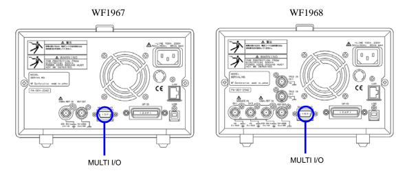
This feature can be used for sweep and sequence control. It outputs the step synchronization code for the sequence.
