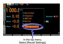
When the MENU key is pressed, the top menu opens. Then, select [Recall Settings]. This opens the Recall Settings screen.
