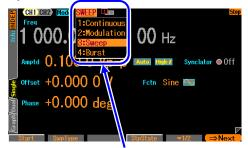
Press the MODE key to open the oscillation mode selection list. Select the sweep oscillation mode [Sweep]. (\*\* P.4-27)
