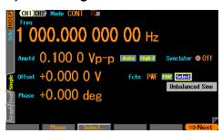
A [Select] button is displayed to the right of the polarity/amplitude range icon when the waveform is set to variable parameter waveform [PWF]. Pressing this button displays the name of the currently selected PWF.
