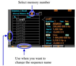
To read source in the built-in memory, press the ENTER key to select the Internal tab.
