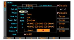
Type: Freq Unit: rpm Form: (h+n)\*m
