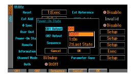
When the Power-On State window opens, select the desired output setting and press the ENTER key.
