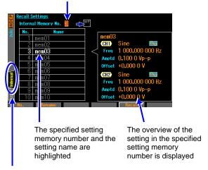
To recall settings saved to the unit's internal memory, select Internal and press the ENTER key.
