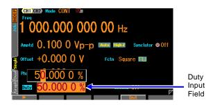
When the [Duty] field is selected and the ENTER key is pressed, the duty input field opens.
