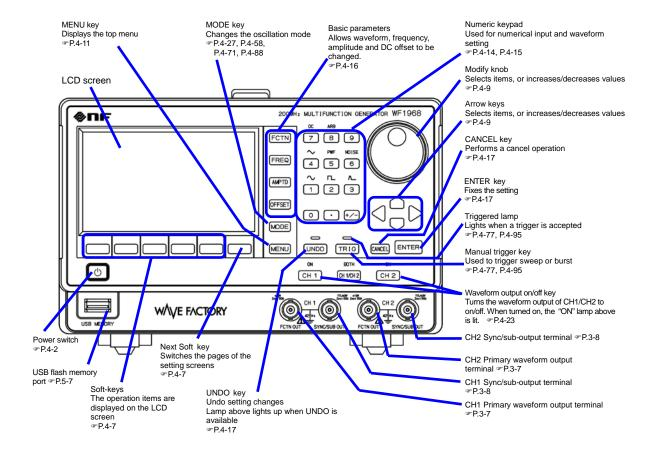
Figure 3-3 Front Panel of WF1968
