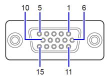
Figure 3-5 Multi-I/O connector pin configuration diagram
