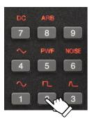
2. Pressing the key directly below the lighting waveform will select that waveform and reflect it in the output. For example, in the image shown to the left, pressing the [2] key will select the Square wave. Another method is to choose the selection list with the arrow keys or modify knob and then press ENTER to apply the settings.
