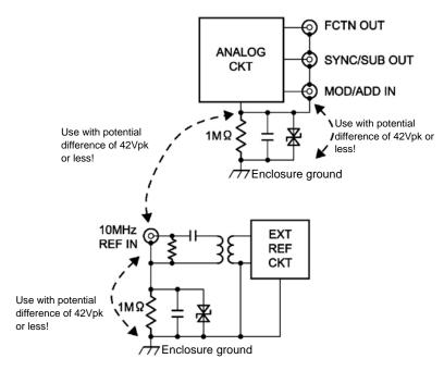
Figure 3-6 Cautions on floating ground connection for WF1967
