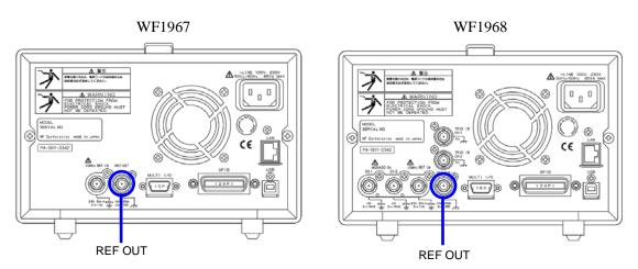
This terminal is used to unify the frequency and phase of multiple WF1967/WF1968 units.
