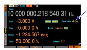
Select [Synclator] and press the ENTER key to turn the Synclator function on or off.
