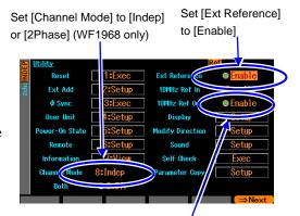
For the connection method 2, set 10MHz Ref Out to [Enable]
