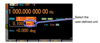
When an input field for each parameter opens, you can change the unit by putting the cursor on the unit at the right end and using the up/down arrow key or the modify knob. The unit name displayed here can be set arbitrarily. Only the display unit is changed without changing the actual output value, when the unit is changed.
