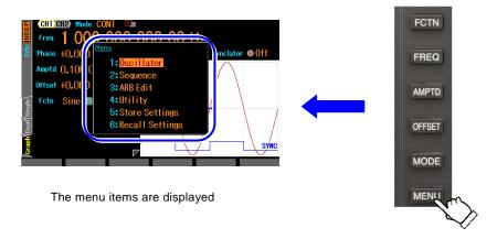
Select the desired item with the arrow keys or the modify knob and then press ENTER key. With the top menu window open, specify the menu item using the numeric keypad [1] to [6].
