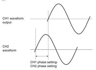
Phase Difference Between Main and Sub Output Can be Changed (Modulation is off or when using External Modulation)
