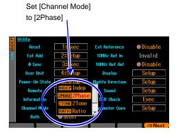
In the Utility screen, set [Channel Mode] to [2Phase] ([Indep] is normally set). This makes the channel mode an oscillation with 2-phase.
