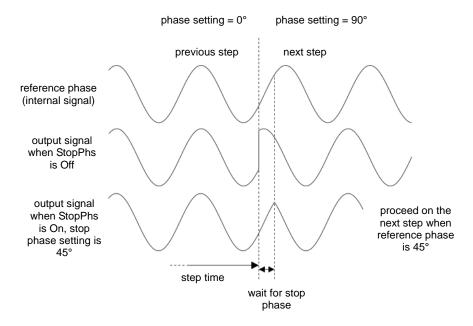
Similarly, following figure show the example, in which the stop phase is a specified and in which it is not specified, when the amplitude is quickly changed.
