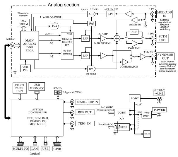
Figure 1-1 WF1967 Block Diagram
