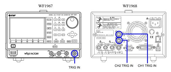
This terminal can be used as external trigger input in the following cases. The polarity setting can be changed.
