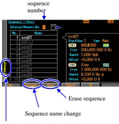
Select Internal tab and press the ENTER key to save to built-in memory
