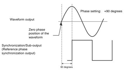
The oscillation start/stop phase is changed in burst Oscillation or gated sweep.
