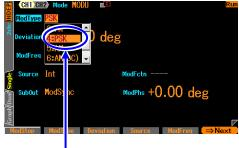
Set the modulation type [ModType] to PSK [PSK] on the second page of the setting screen when the oscillation mode [Mode] is set to modulation [MODU] and on the third page of the setting screen when the mode is sweep [SWEEP].
