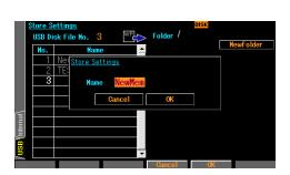
2. When saving to USB, first connect the USB flash memory to the unit, then select the USB tab on the far left of the screen and press the ENTER key. In the Store Settings screen, select the [USB Disk File No.] field on the top left of the screen, and then press the ENTER key to open the input field of the setting memory number to be saved. Use the up/down arrow keys or the modify knob to increment or decrement the setting memory number.
