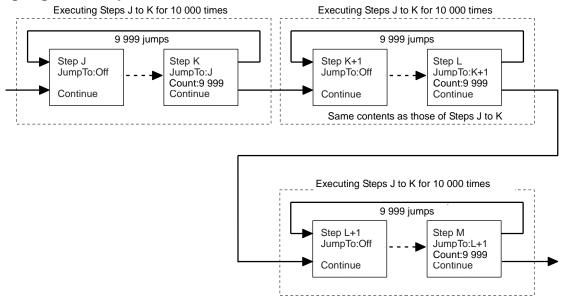
Steps with the same contents can be created easily by using the [Copy] and [Paste] soft keys. Create the steps with the same contents and then revise only the required portions.
