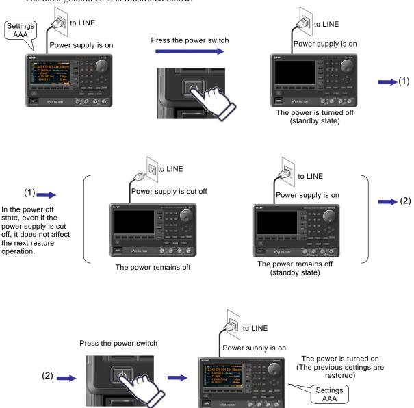
While the power is off, if the power supply is cut off due to the disconnection of the power cord or the shutoff of the connected breaker, this does not affect the restore operation the next time
