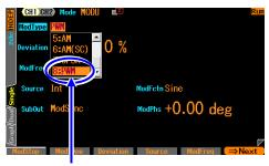
Set the modulation type [ModType] to PWM [PWM] on the second page of the setting screen when the oscillation mode [Mode] is set to modulation [MODU] and on the third page of the setting screen when the mode is burst [BURST] or sweep [SWEEP].
