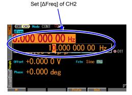
In the Oscillator screen, set the frequency difference in  $[\Delta Freq]$  of channel 2. The frequency of channel 2 results from adding this frequency difference to the frequency of channel 1.
