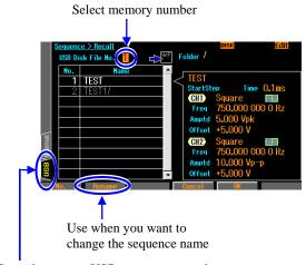
To read source to USB memory, press the ENTER key to select [USB] tab
