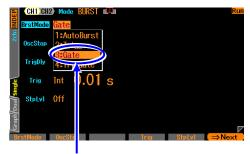
the second page of the setting screen, and press the ENTER key to display the burst mode selection list. Selecting gate oscillation [Gate] sets the gate oscillation mode.
