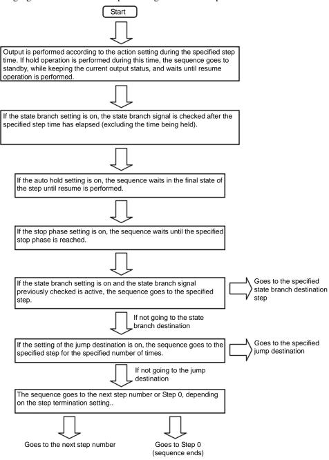
Following transitions occur as the result of event branching or termination operation, regardless of the flow in the step.
