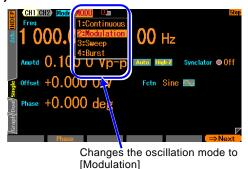
Press the MODE key to open the oscillation mode selection list. Please select the modulated oscillation mode [Modulation]. (\*\* P. 4-27)
