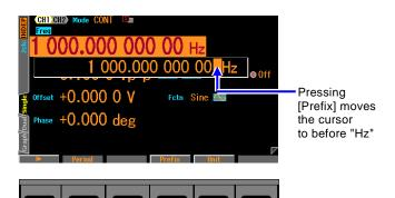
Press the [Prefix] soft-key to move the cursor to before "Hz".
