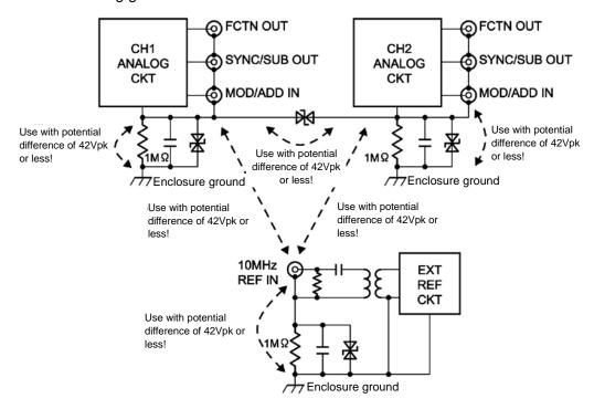
Figure 3-7 Cautions on floating ground connection for WF1968
