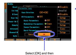
4. When the above setting is completed, select [OK] at the bottom of the window, and then press the ENTER key. The copy operation is performed. When you do not want to copy, select [Cancel] at the bottom of the window and press the ENTER key, or press the CANCEL key.
