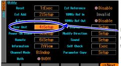
In the Utility screen, select the [User Unit] field and press the ENTER key.
