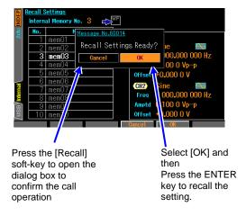
Press the [Recall] soft-key to open the dialog box to confirm the recall operation.
