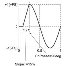
The amplitude of the original Sine wave is fixed at  $\pm FS$ . Please note that the amplitude may be less than  $\pm FS$
