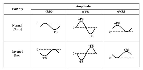
"Reverse" only reverses a waveform without changing the sign of output DC offset.
