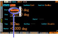
When the oscillation mode [Mode] is set to sweep oscillation mode [SWEEP], select the sweep type [SwpType] on the second page of the setting screen to display the selection list. Selecting phase [Phase] sets the phase sweep.
