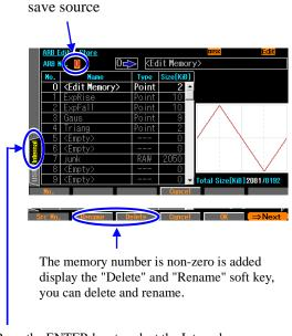
Press the ENTER key to select the Internal tab to save source to edit memory.
