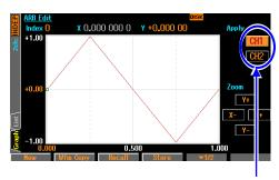
When you press the Apply button, waveform in process of creation is output.
