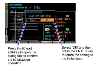
As with the save operation, press the [Clear] soft-key after setting the setting memory number. The dialog box to confirm the initialization operation is opened.
