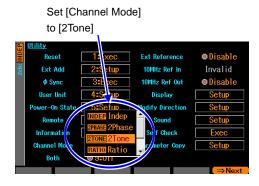
In the Utility screen, set [Channel Mode] to [2Tone] ([Indep] is normally set). This makes the channel mode an oscillation with constant frequency difference.
