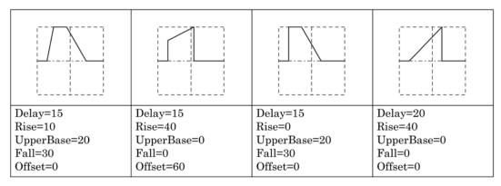
The amplitude direction offset of the entire trapezoid. Variable range: 0.00% to 100.00%
