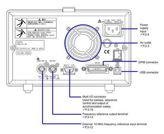
Figure 3-2 Rear Panel of WF1967
