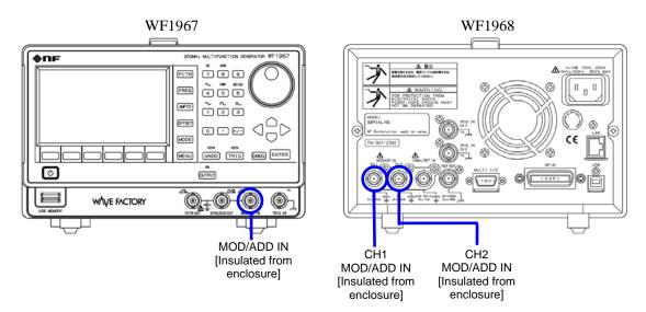
When the modulation source is external in the modulation mode except FSK and PSK, an external modulation signal is input. In the FSK or PSK modulation mode, the external trigger input is used as external modulation signal input.
