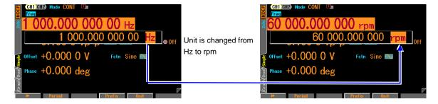
This can display and set a value in units of rpm.
