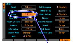
In the Utility screen, select [φSync] and then press the ENTER key to execute the phase synchronization
