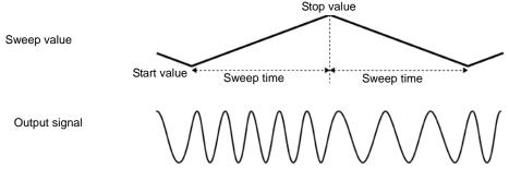
When the phase increases, the frequency rises as by the following value. When the phase decreases, the frequency falls by following value.
