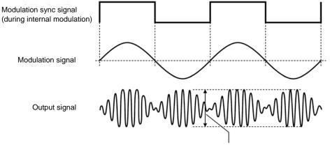
Amplitude setting value (Vp-p) x Modulation depth (%)/100
