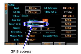
Select the external control interface from USB, GPIB or LAN(option).
