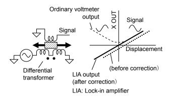
Good linearity bidirectional position detection can be performed using phase detection. This is also suitable for position feedback control.
