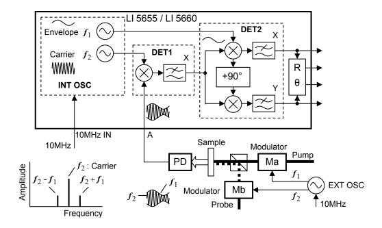
Envelope information can be obtained by detecting the amplitude modulation signal.
