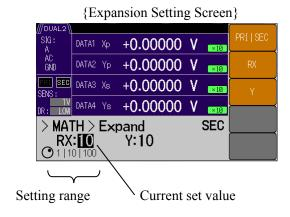
Press the [MATH>] soft key to go to the {Math Selection Screen}. Select EXPAND using the MODIFY knob or up/down keys to display the [EXPAND>] soft key.
