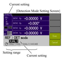
Press the [DET MODE>] soft key from the {Reference Signal Setting Screen} to go to the {Detection Mode Setting Screen}.
