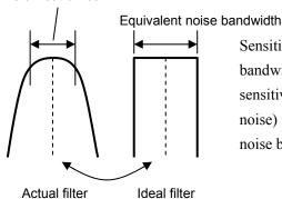
Sensitivity to white noise is represented by an equivalent noise bandwidth. The bandwidth of an ideal filter where the sensitivity to noise (in other words, the RMS value of output noise) is equal to that of the actual filter is called an equivalent noise bandwidth of that filter.
