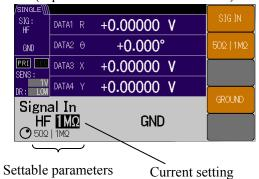
If the frequency exceeds 1 MHz and the reflection of the signal cannot be ignored, it is recommended to set both the characteristic impedance of the connection cable and the input impedance of the HF connector to  $50~\Omega$ .
