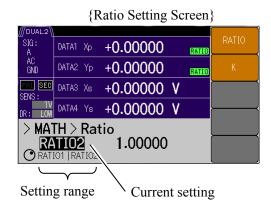
detection mode is DUAL1 or DUAL2, secondary PSD output (Xs) can be specified as the numerator, in addition to the normal AUX IN.
