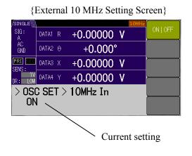
Next press the [OSC SET>] soft key to go to the {Internal Oscillation Setting Screen}.
