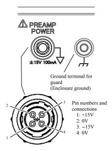
If you do not need in particular a low noise, power can be supplied to the preamplifier from the PREAMP POWER connector on the rear panel of the LI5655 / LI5660.
