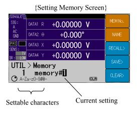
To change the setting memory name, press the [NAME] soft key to move through the positions using the left/right cursor keys and then set the memory name (1 to 8 characters) using the MODIFY knob or up/down keys.
