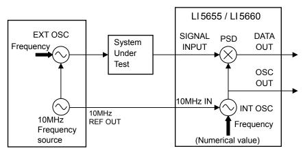
Figure 5-2 10 MHz Synchronous System Example
