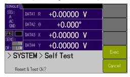
First, press the UTIL key to move to the {Utility Screen}, then press the [SYSTEM>] soft key to go to the {System Setting Screen}, then press the [SELF TEST>] soft key to go to the {Self Diagnosis Screen}.
