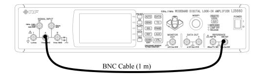
Connect the OSC OUT and the "A" of SIGNAL INPUT with a BNC cable (1 m).
