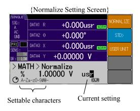
Press the [USER UNIT] soft key to move through the digits using the left/right cursor keys and set the user unit string (1 to 3 characters) using the MODIFY knob or up/down keys.
