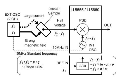
If the original frequency is an integer ratio, the difference frequency signal can also be measured using the fractional harmonic measurement function. Both can avoid a crosstalk interference from the external reference signal.
