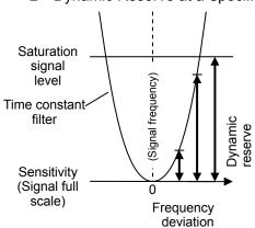
The dynamic reserve value depends on the saturation signal level inside the device at a specific sensitivity (signal full scale) and the characteristics of removing noise using the time constant filter. In other words, it depends on the frequency.
