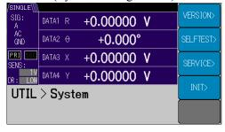
Press the [SYSTEM>] soft key to go to the {System Setting Screen}.
