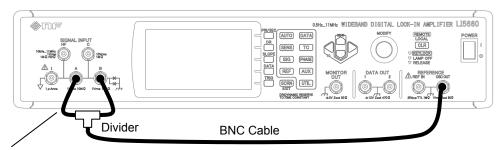
Two short BNC cables with the same characteristics
