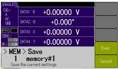
To save the setting to the setting memory selected in the {Setting Memory Screen}, press the [SAVE>] soft key. The confirmation screen is displayed. To execute it, press the [Exec] soft key, and to cancel it, press the [Cancel] soft key.
