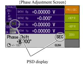
Press the [ PRI | SEC ] soft key to switch between the primary PSD and secondary PSD settings.
