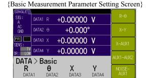
Next, press the [BASIC>] soft key to go to the {Basic Measurement Parameter Setting Screen}, where the basic combination soft key is displayed.
