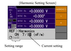
To set the harmonic measurement, first press the REF key to go to the {Reference Signal Setting Screen}.
