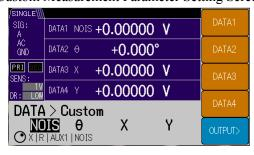
Press the [CUSTOM>] soft key and then the [DATA1] soft key to select "NOIS" using the MODIFY knob or up/down keys. NOISE is set in DATA1. (Other settings are not changed.)
