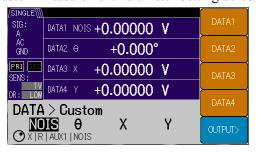
Press the [CUSTOM>] soft key and then the [DATA1] soft key to select "AUX1" using the MODIFY knob or up/down keys.
