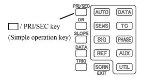
constant (TC), and attenuation slope (SLOPE) of the PSD that is lit can be set.
