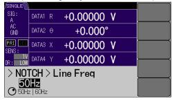
The line frequency (fundamental) can be selected from {50Hz | 60Hz}.
