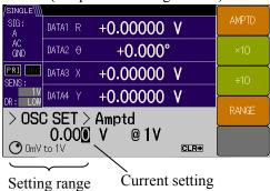
Press the [AMPTD>] soft key to go to the {Amplitude Setting Screen} and set the amplitude using the cursors and MODIFY knob.
