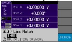
The line filter function (removal frequency) can be selected.
