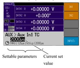
Press the [AUX IN>] soft key from the {Auxiliary I/O Setting Screen} to go to the {Auxiliary Input Setting Screen}.
