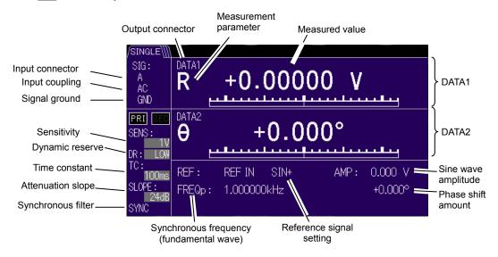
Note that the display can be switched to the expanded display and details display using the SCRN key.
