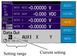
If you return to the {Output Signal Setting Screen}, the [NOISE] soft key is displayed.
