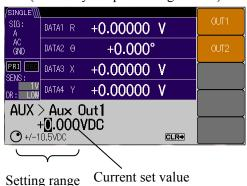
Press the [AUX OUT>] soft key from the {Auxiliary I/O Setting Screen} to go to the {Auxiliary Output Setting Screen}.
