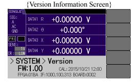
Displays the firmware version and last adjustment date and time.
