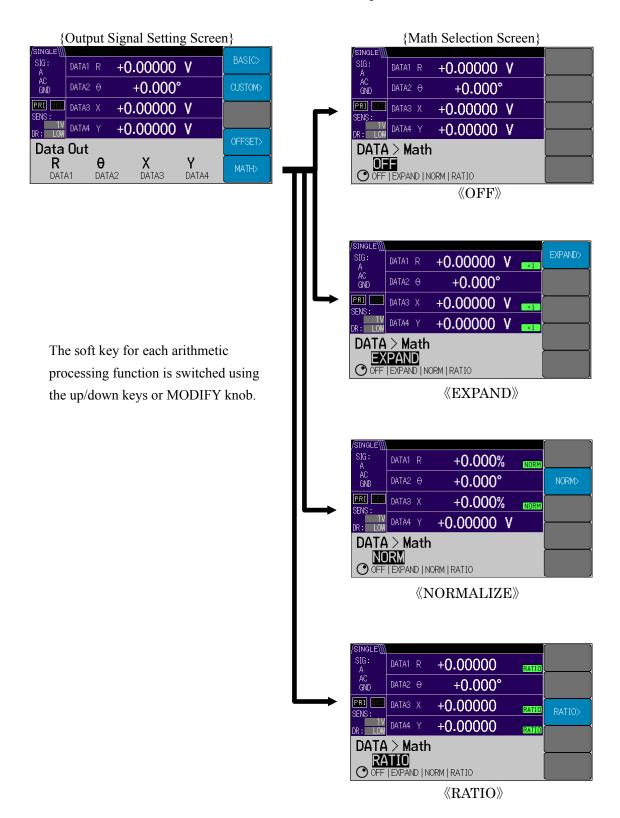
During each arithmetic function, When you press the [MEASURE] soft key or the [SENS] soft key of the AUTO key {Auto Setting Screen} or the [AUTO] soft key of the SENS key {Sensitivity Setting Screen}, the arithmetic processing function is canceled.
