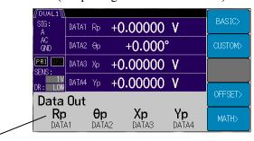
Current DATA1, DATA2, DATA3, DATA4 output and display parameters (for DUAL1)
