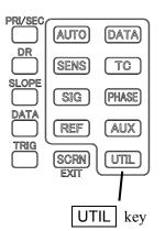
To view the {Maintenance Information Screen}, press the UTIL key to display to the Utility Screen.
