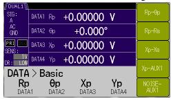
Next press the [BASIC>] soft key to display the basic combination of soft keys.
