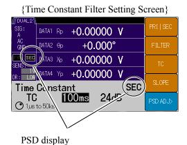
To set the time constant, first press the TC key to go to the {Time Constant Filter Setting Screen}.
