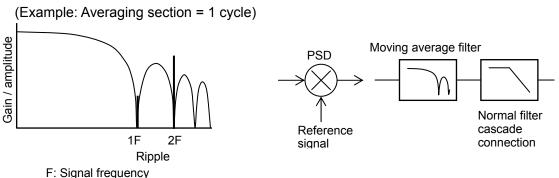
If you need a high-speed response, set 6 dB/oct for the attenuation slope. However, the output waveform looks slightly like a series of steps.
