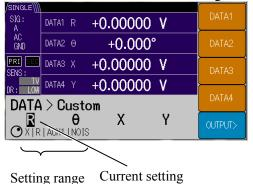
Press the [CUSTOM>] soft key to go to the {Custom Measurement Parameter Setting Screen}, where any measurement parameter can be set in DATA1 to DATA4.
