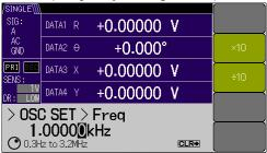
The frequency for the internal oscillator can be set. The setting range varies depending on the input signal connector.
