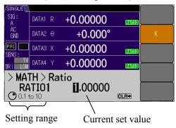
Press the [K] soft key in the {Ratio Setting Screen} to move through the digits using the left/right cursor keys and then set the K constant using the MODIFY knob or up/down keys.
