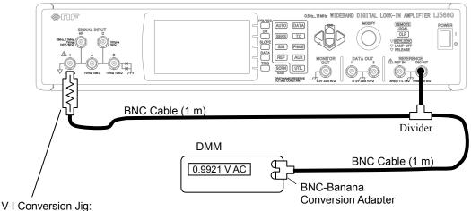
Uses a resistor of precisely known value.
