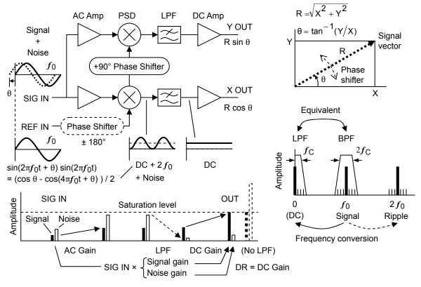
Figure 1-1 Basic Principle of a Lock-in Amplifier
