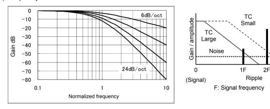
Normalized frequency = |frequency difference from signal to reference| / cutoff frequency (fc) fc = 1 / ( $2\pi T$ ), T indicates the time constant.
