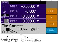
Press the [FILTER] soft key to set the normal filter (TC filter) and SYNC (synchronous filter) using the MODIFY knob or up/down keys.
