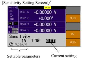
Press the [AUTO] soft key to set HOLD or AUTO for the auto sensitivity adjustment using the MODIFY knob or up/down keys.
