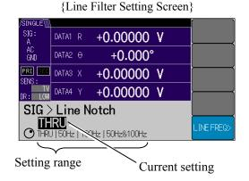
Next press the [LINE NOTCH>] soft key to go to the {Line Filter Setting Screen}.
