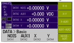
To display the noise density, press the [BASIC>] soft key and then the [NOISE-AUX1] soft key. NOISE and AUX IN 1 are set in DATA1 and DATA2, respectively. (Other settings are not changed.)
