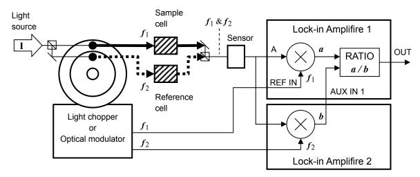
Figure 5-3 Ratio Measurement Application Example (Dual Beam Method)
