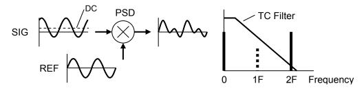
If a large DC component is included in the input signal, set AC for the input coupling.
