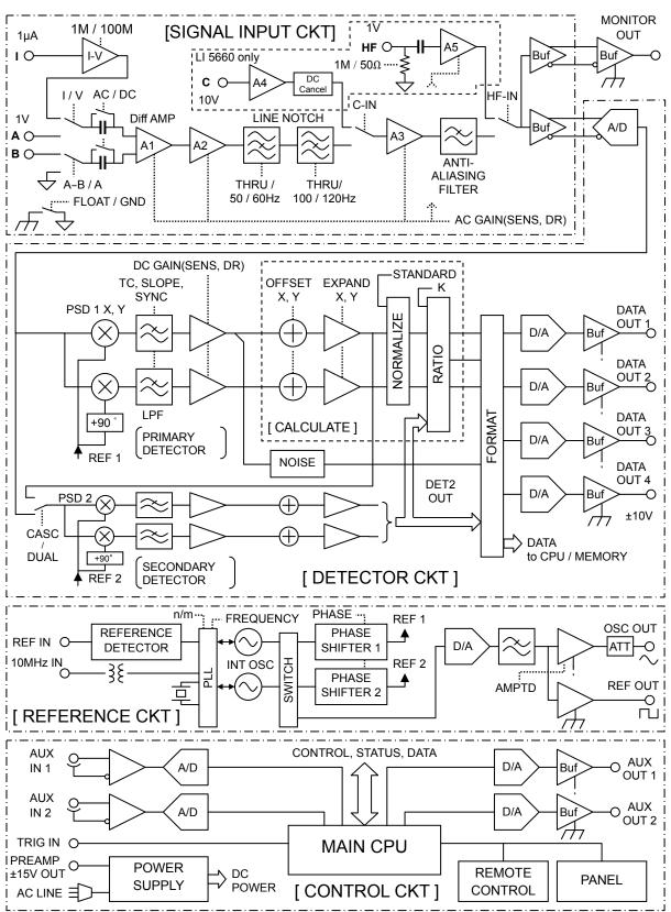
Figure 1-2 LI 5655 / LI 5660 Block Diagram
