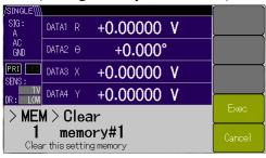
To clear the setting memory selected in the {Setting Memory Screen}, press the [CLEAR>] soft key. The confirmation screen is displayed. To execute it, press the [Exec] soft key, and to cancel it, press the [Cancel] soft key.
