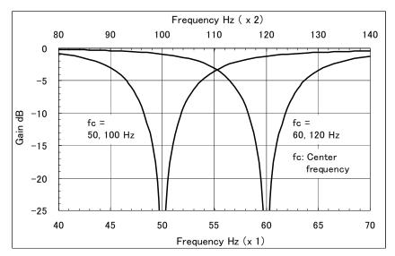
Figure 5-1 Line Filter Characteristics
