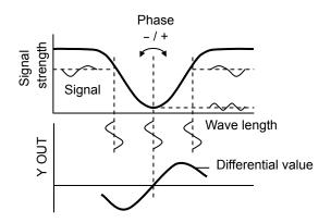
If a minute "change" is superimposed on the wavelength sweeping and the "change" of the signal strength is measured using a lock-in amplifier, the differential value of the characteristic curve can be obtained. This value goes through zero at the peak or bottom of the characteristic curve (a positive/negative inversion occurs), so it is easy to obtain that position.
