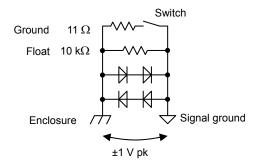
The ground impedance between the signal ground and enclosure can be switched between float and ground. If a voltage exceeding  $\pm 1$  V is applied, this isolation cannot be maintained.
