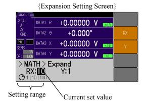
Next press the [ MATH> ] soft key to go to the {Math Selection Screen} Select "EXPAND" using the MODIFY knob or up/down keys
