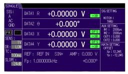
When the offset function is set to ON, the "OFS" icon is displayed in the measurement data field.
