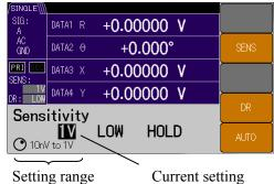
Press the [ SENS ] soft key to set the sensitivity using the MODIFY knob or up/down keys.
