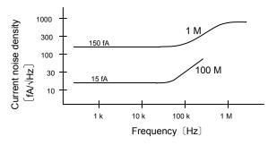
Figure 4-4 I Input Referred Noise Density (Supplementary Values)
