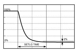
Response characteristics (for the continuous auto adjustment operation)
