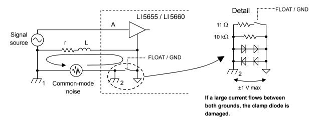
If the signal source is not grounded, select GND and connect the signal ground to the enclosure of the LI5655 / LI5660 to maintain the stability of the potential reference.
