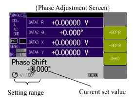
When you enter the operation screen, you can move through the digits using the left/right cursor keys and then set the numerical value using the MODIFY knob or up/down keys.
