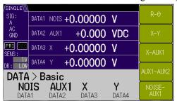
Press the [BASIC>] soft key and then the [AUX1-AUX2] soft key.
