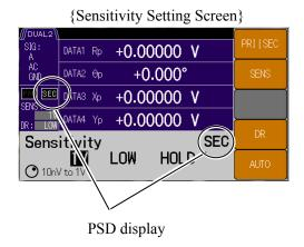
Press the [PRI | SEC] soft key to switch between the primary PSD and secondary PSD settings.
