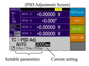
Press the [AUTO] soft key from the {PSD Adjustment Screen} to select AUTO or HOLD in the continuous auto setting using the MODIFY knob or up/down keys.
