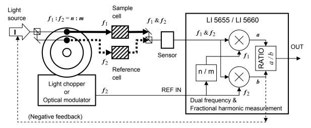
To avoid mutual interference, avoid two frequencies from being in a relationship of harmonic and subharmonic. Modulation and detection are also possible by two arbitrary frequencies by synchronizing with an external signal generator using the 10 MHz synchronization function.
