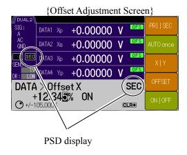
Press the [OFFSET>] soft key to go to the {Offset Adjustment Screen}.
