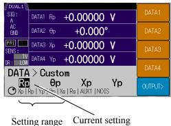
Press the [ CUSTOM> ] soft key to arbitrary set parameters in DATA1 to DATA4.
