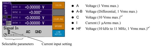
Connect the cable to the selected input connector.
